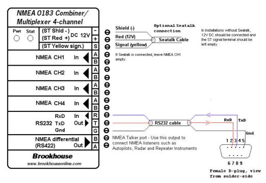
1. Choose a location where you will install your NMEA Multiplexer. The NMEA multiplexer (with or without repeater display) is usually placed in the vicinity of the boat's nav-station, close to the computer. Please note that both the multiplexer itself and the display are not waterproof, they should not be installed in the boat's cockpit but inside the cabin at a dry, protected location. Avoid connecting sensitive electronics to the same battery(-bank) as electric winches, start-motors etc.
